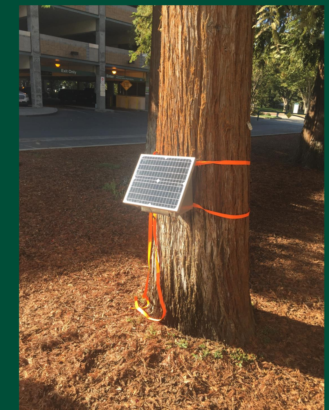
Figure 4: Deployable sensor mounted to a tree.
